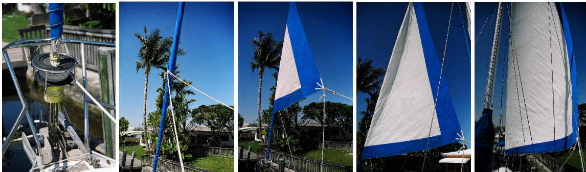
FIGURE 15-3 UNFURLING A ROLLER REEF HEADSAIL
