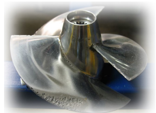
FIGURE 13-8 CORRODED PROP DUE TO CAVITATION
