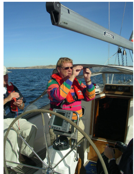
FIGURE 19-19 TAKING BEARING WITH HANDHELD COMPASS
