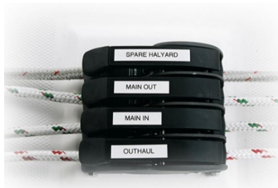
FIGURE 15-11 LOCKING CLEATS OR ROPE CLUTCHES
