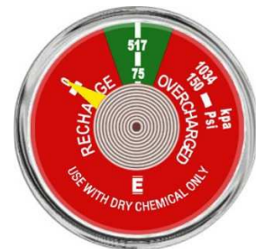
FIGURE 3-8 FIRE EXTINGUISHER GAUGE
