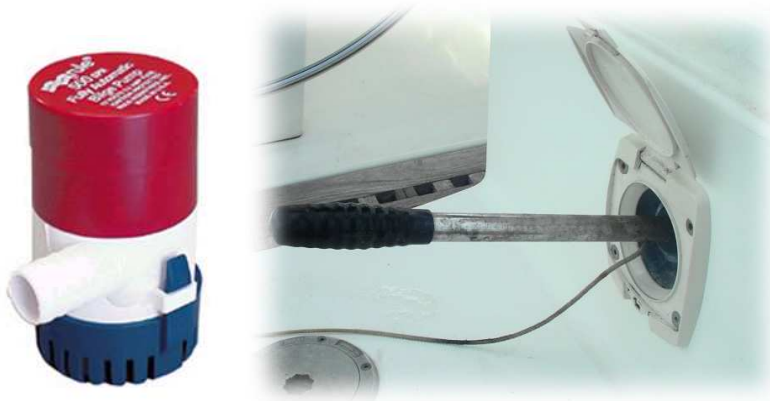
FIGURE 1-64 ELECTRIC &amp; MANUAL BILGE PUMPS
