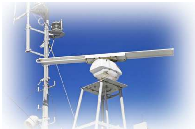
FIGURE 1-91 SPINNING RADAR DOME
