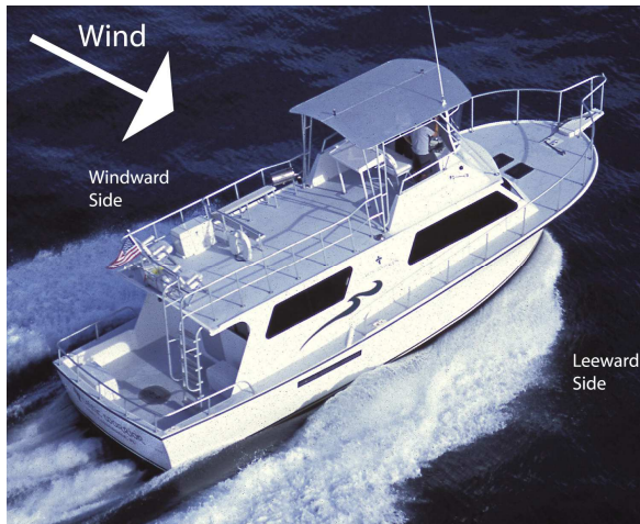
FIGURE 1-93 WINDWARD & LEEWARD - POWER
