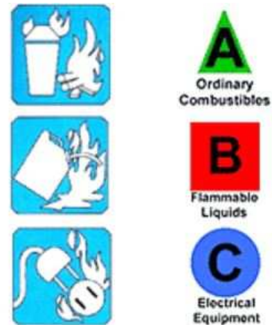
FIGURE 3-7 FIRE RATING SYSTEM
