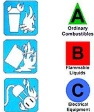
FIGURE 3-7 FIRE RATING SYSTEM
