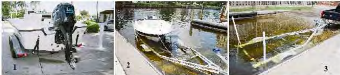
FIGURE 12-16 TRAILER LAUNCH SEQUENCE
