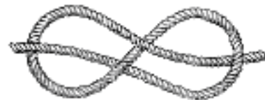
FIGURE 5-3 FIGURE OF EIGHT KNOT
