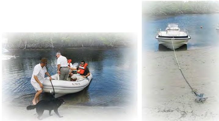
Kill engine and coast to beach, crewmember to pull line & anchor/boat to beach, secure anchor onto beach.
