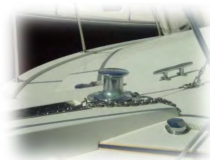
FIGURE 1-56 WINDLASS FOR HAULING ANCHOR
