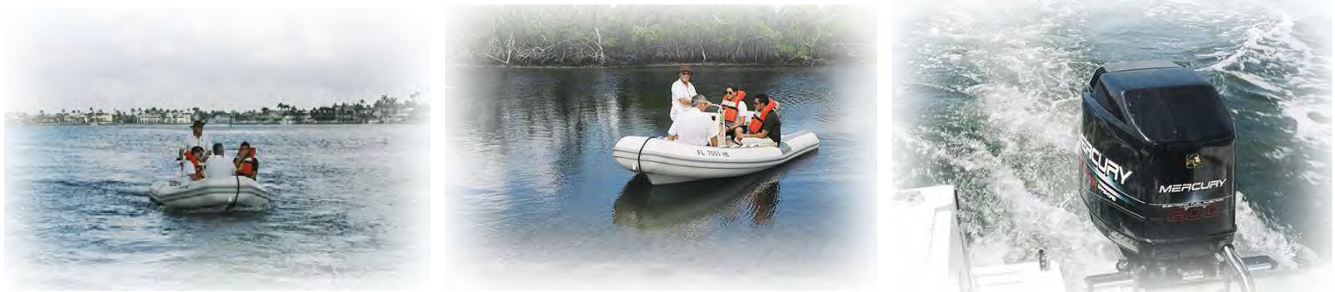
Approach with controlled speed, someone at bow as lookout, tilt outboard engine up 1/3
