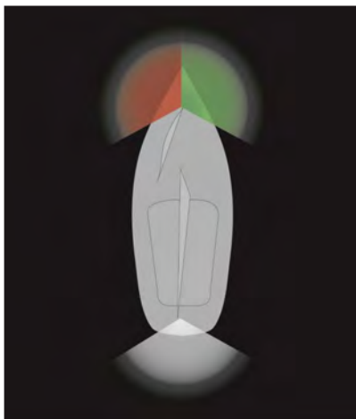
FIGURE 21-17 SBT 20M AND OVER
