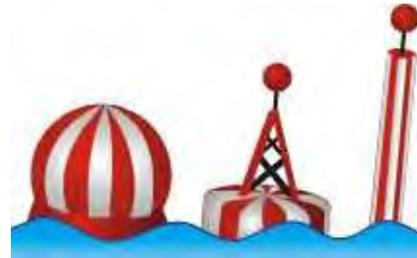
FIGURE 19-6 SAFE WATER MARK
