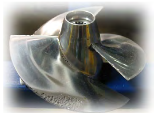
FIGURE 12-8 CORRODED PROP DUE TO CAVITATION
