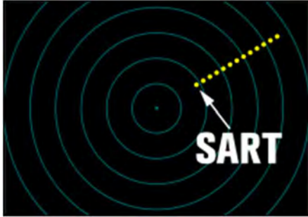
FIGURE 2-16 A MOCK-UP RADAR TRACE FROM SART
